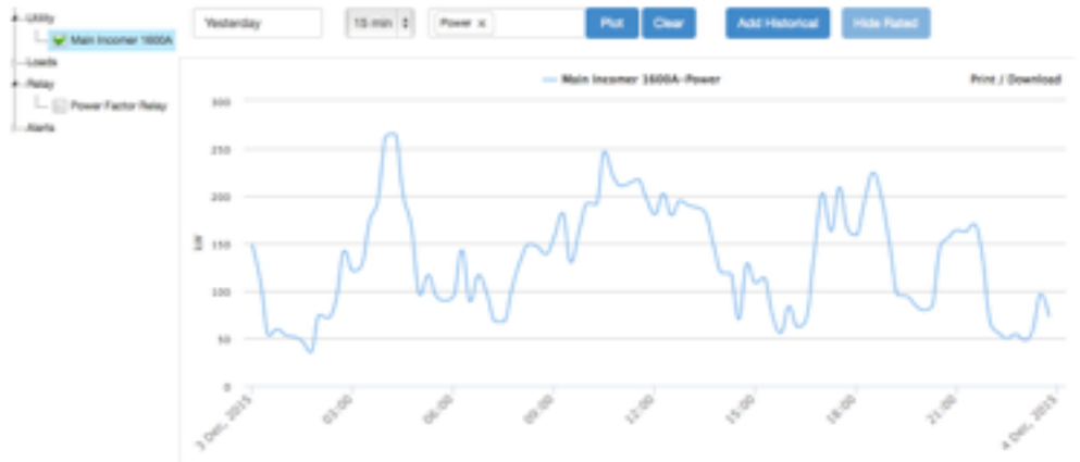
Energy Consumed in Selected Period Main Incomer 1600A : 3132 kWh
